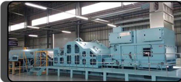
HOPPER FEEDER & CARDING M/C – BKCD MACHINE
